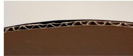
Cardboard is made with structural channels called flutes which create this wavy shape in between layers.
