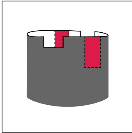
Remove the plastic protective film from microscope slides. Place one slide into the deeper notches. You now have your microscope slides set on a stage to view your samples.
